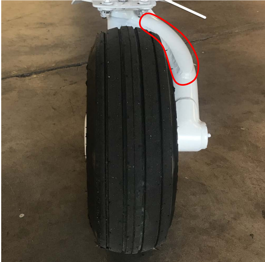
Figure 45-1g Custom Air 94130-9 with reinforcement strap pictured. 94130-1 and -5 do not have reinforcement strap.
